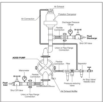
separated from the fluid by a membrane called a diaphragm. The diaphragm in turn applies pressure on the fluid and forces it out of the pump discharge. While this is occurring, the opposite air chamber is depressurized and exhausted to atmosphere and fluid is drawn into the pump suction. The cycle again repeats, thus creating a constant reciprocating action which maintains flow through the pump. The flow is always in through the bottom suction connection
