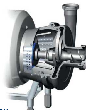
Special version equipped with an inducer in the suction port. This device is fitted immediately upstream of the impeller to reduce the NPSH required by the pump.
