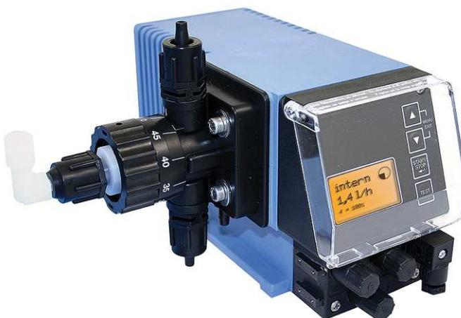
All metering pumps of the series ELADOS® EMP-KKS operate on the piston-diaphragm principle. The diaphragm serves to feed the product whereas the piston handles the metering. Because of the continuous surplus return this metering pump operates self-venting. Therefore, the pump is appropriate for the conveying of degassing products. The cylindrical piston system without seal
