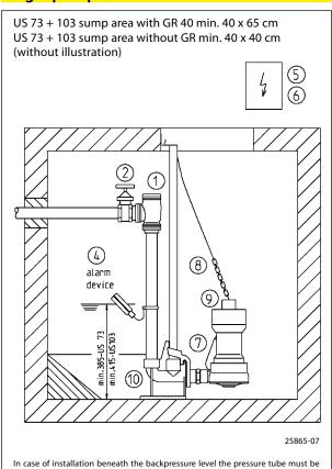
taken in a loop over the local backup level acc. to EN 12056. Besides, it must be secured with a EN 12050-4-proofed swing-type check valve. Additionally we recom-
