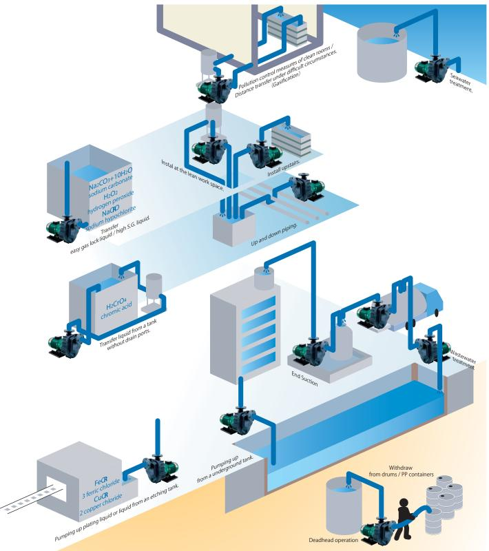
• Possible to install it far from a tank or filter. • Stringent instal condition has a great reduction. • Up and down suction piping is possible. • No need foot valves.
