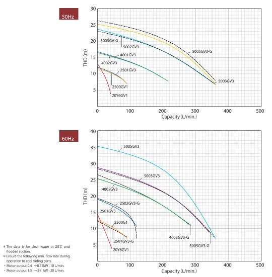
**GVF** series (Main material: CFR ETFE)
