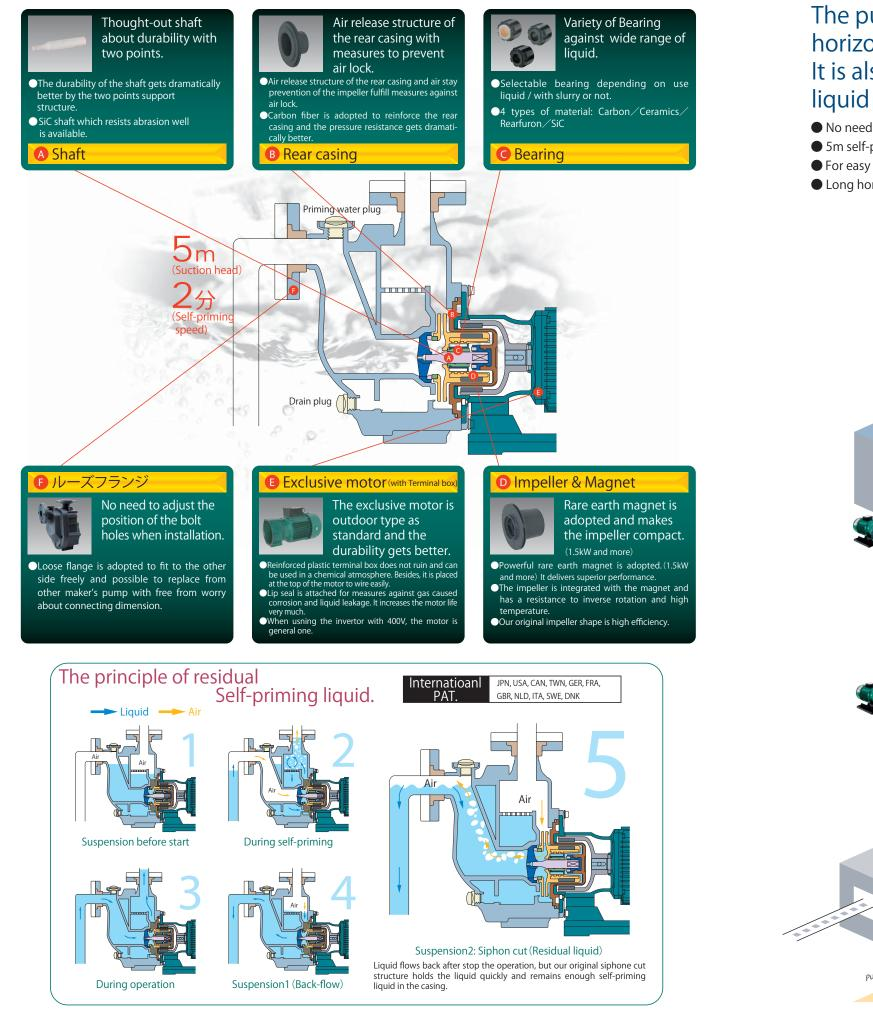
The pump can be used for all types of installation site such as horizontal suction piping or under stringent conditions. It is also effective to take measures against earthquakes or liquid leakage.
