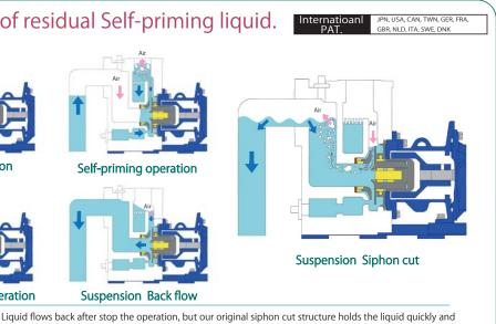
remains enough self-priming liquid in the casing. Therefore, it is not necessary to pour priming liquid after
