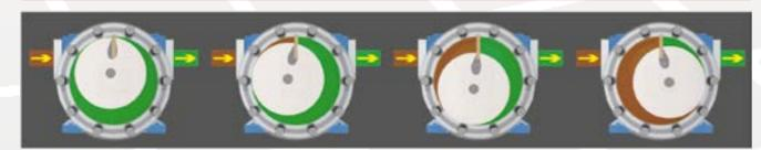
The hollow disc is eccentrically mounted in the rotor shaft and turns around the suction and discharge cameras separator vane. In this way the piston is obliged to follow the trajectory around the vane and externally to the pump head, where it is pushed via an elastic device internally inserted.
