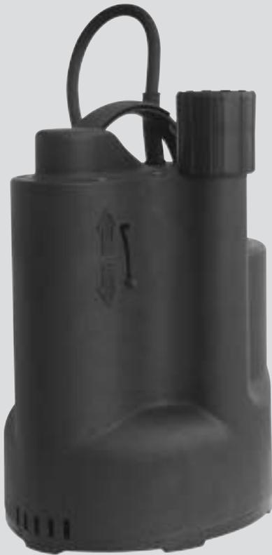
The DPC pump has been designed for domestic applications as drainage of seepage water, pumping of water from sump pits, water deposits or collection tanks. Equipped with rubber holder for 3/4 or 25-32 Ø hoses and check valve.
